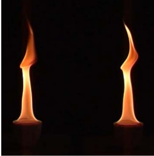
Figure 4. Screenshot of synchrony pulsing diesel pool fires: pure (left) and with 1% ferrocene (right)
