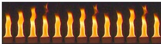
Figure 1. Diesel pool fire (40 mm diameter) with periodic ascending flame structures received with 50 fps.
