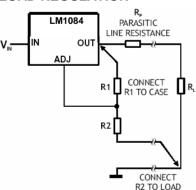
True remote load sensing it is not possible to provide, because the LM1084 is a three terminal device. The resistance of the wire connecting the regulator to the load will limit the load regulation.
