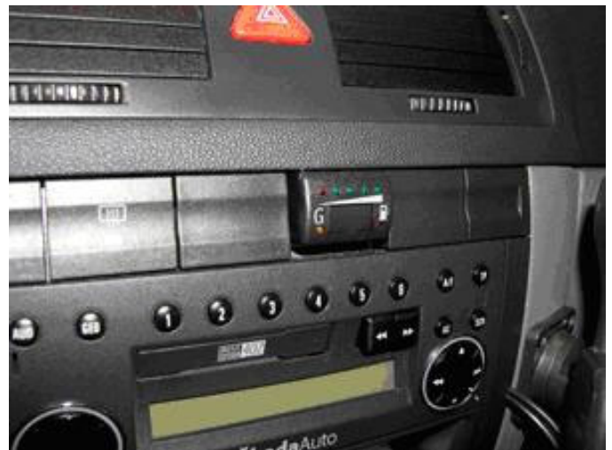
The LED dashboard display of CNG level
