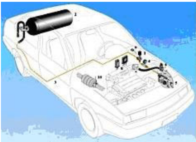
The CNG system in a dual fuel car
