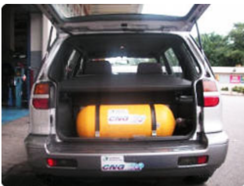
The CNG cylinder in the trunk
