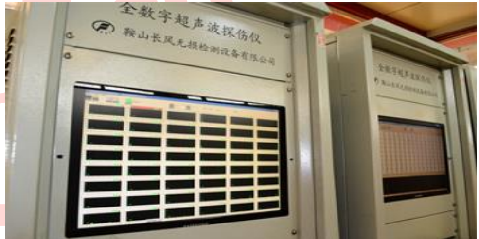
Continuous Monitoring Equipment of Ultrasonic Flaw Detection
