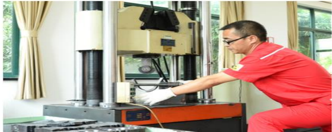
Tensile Test (Microcomputer-controlled Electro-hydraulic Servo Universal Testing Machine)
