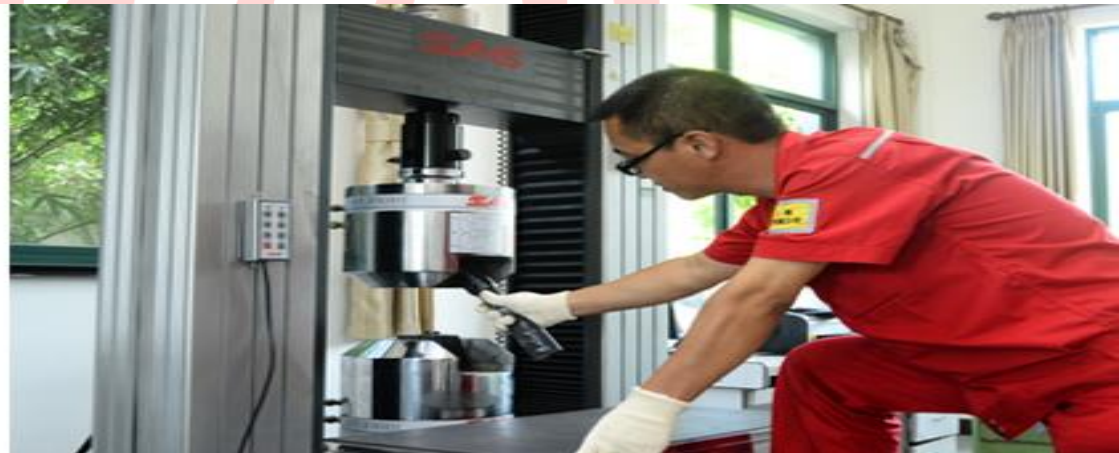
Tensile Test (30-ton Electronic Universal Testing Machine)
