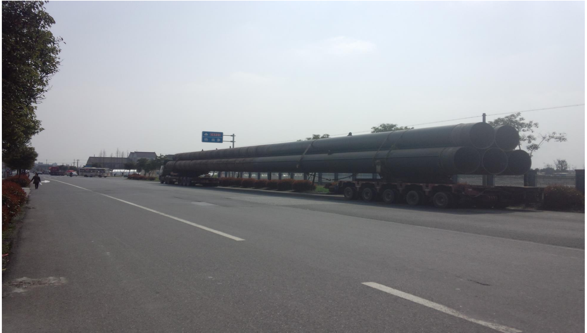
TRUCK TRANSPORTED EXTRA LENGTH PIPE PILING
