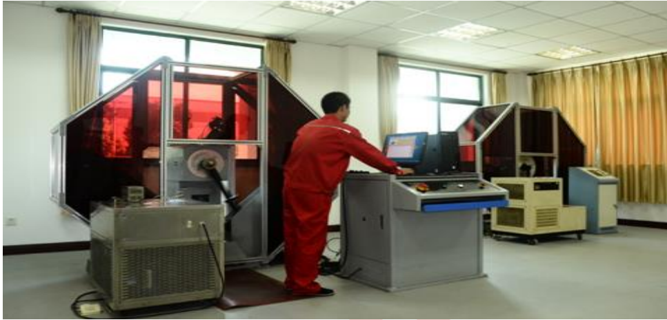
Impact Test (500J Impact Testing Machine)
