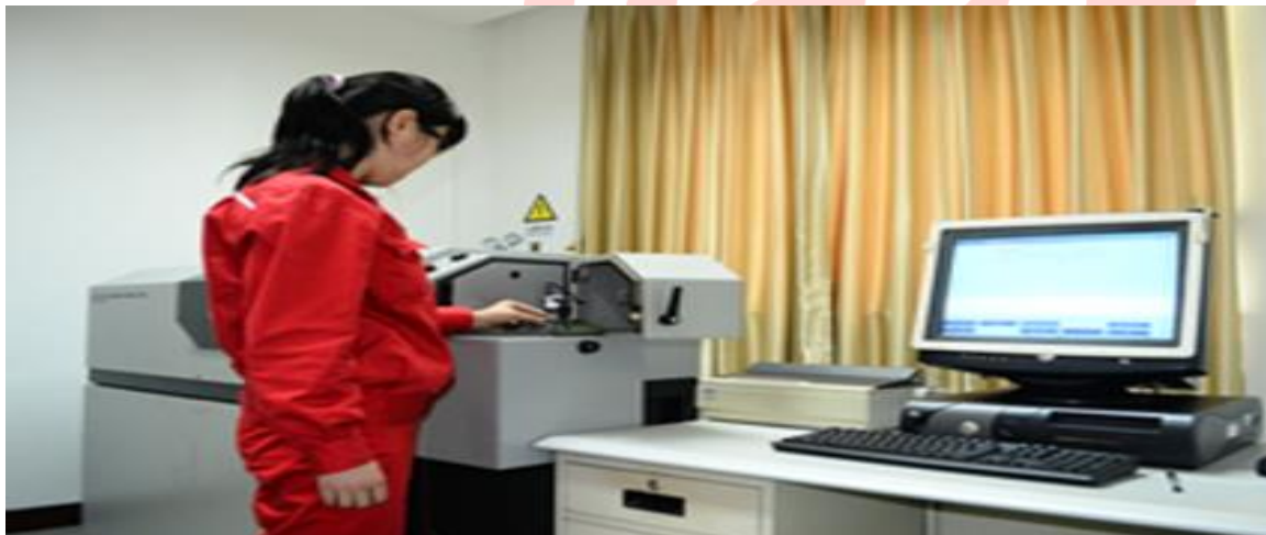
Spectrographic Analysis Test (Direct-reading Spectrometer)
