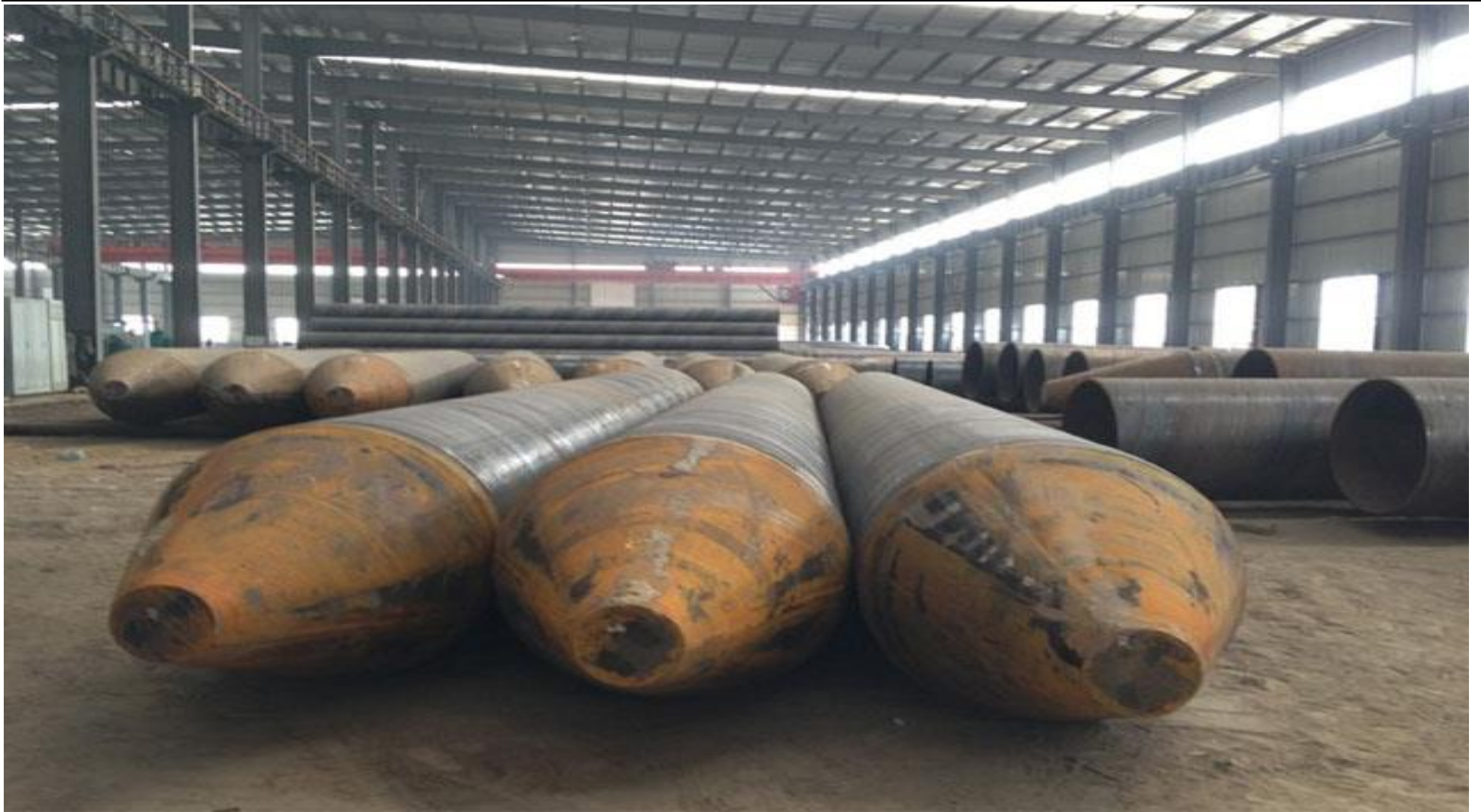
PIPE PILING WITH DRIVING SHOES
