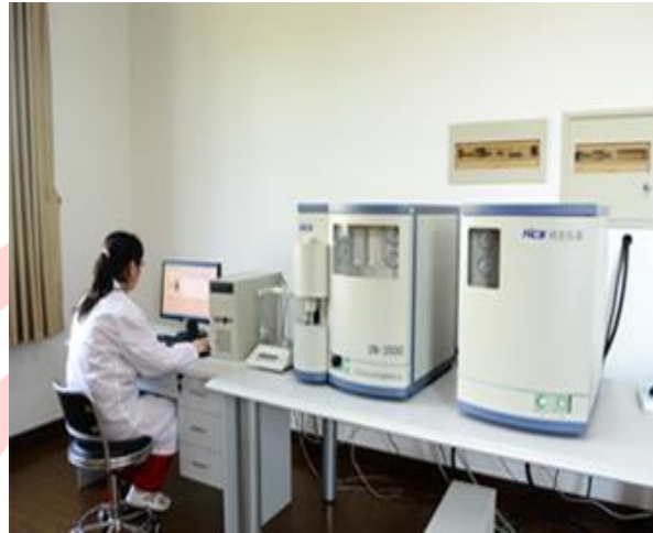
Nitrogen Test (Oxygen/Nitrogen Determination)
