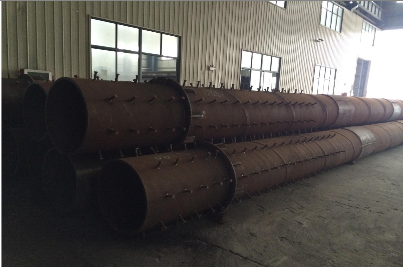
AS1163 C350L0 STUBBED PIPE PILING
