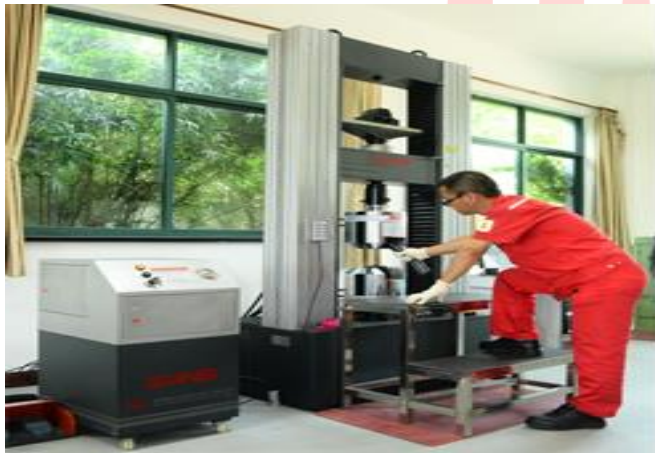
Tensile Test (Microcomputer-controlled Electro-hydraulic Servo Universal Testing Machine)
