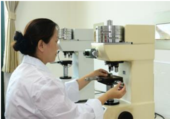
Hardness Test (Small-load Vicker Hardness Testing Machine)
