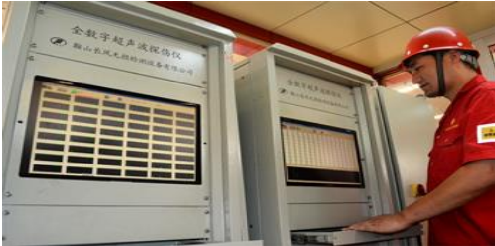
Continuous Monitoring Equipment of Ultrasonic Flaw Detection
