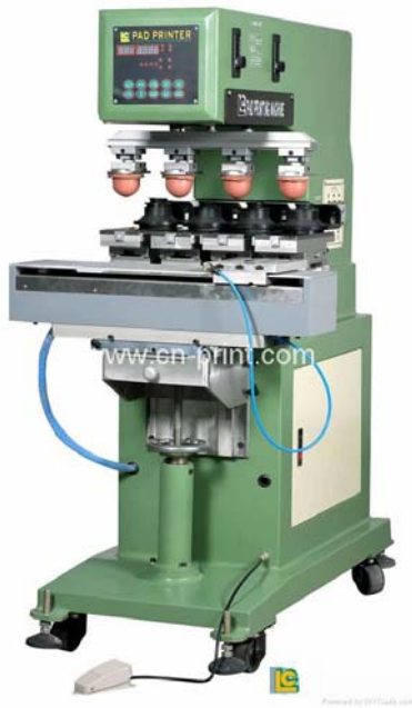
Figure 3: 4-color pad printer with shuttle & sealed ink cup made by Luen Cheong Printing Equipment Group Limited.
