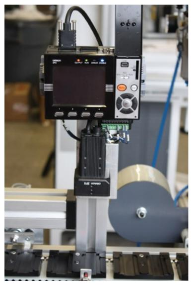
A High-Tech Helper: This automated inspection system, installed above the just-printed parts, measures print registration and opacity—an integral part of manufacturing precision medical products.
