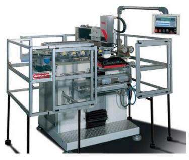
Custom Solutions: Presses, such as the one shown here, can be customized for a wide variety of industrial uses, including decorating a panel that requires several different pads to print the different images in different locations. Programmable pad printers can store an unlimited number of print parameters, which can be called up or edited, depending on the shape and style of panel being printed.
