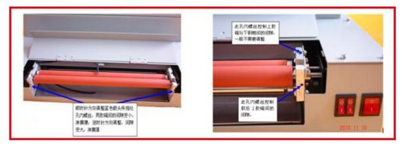
7) If not to use the machine for long time, you'd better clear rubber rollers before you store it. Pull the alcohol into the storage tank to replace the glossy oil, and keep the machine working for a while. Or open the cap of the rubber roller, pull the alcohol between the 2 rollers, keep the rollers work for a while, or use a piece of cotton with alcohol clean the rubber roller.
