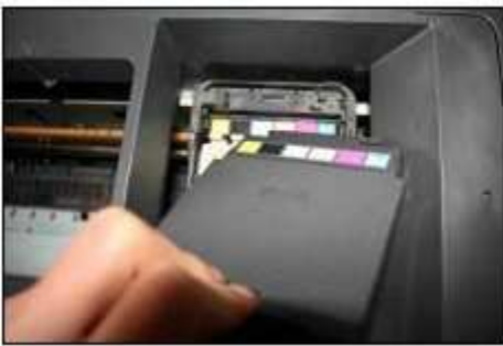
Then remove the cartridge cover directly
