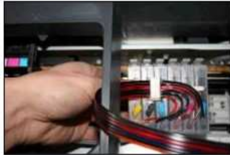
Place the cartridge and pipeline though the printer cover as above picture shown
