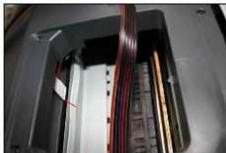
The clip along the bottom side of the printer cover
