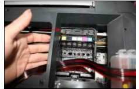
Then move the carriage to the right-side
