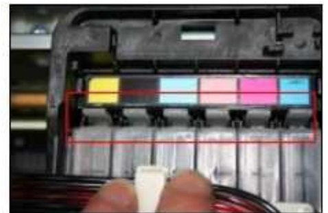
As the red rectangle shown, if all the cartridges are well installed, there will be a little sound
