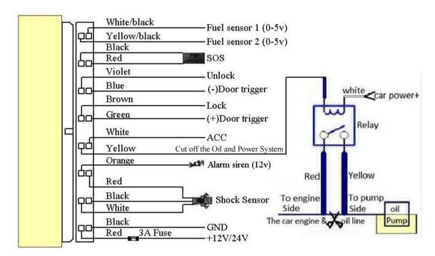
Wiring diagram of central locking system's relay:
