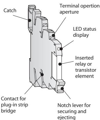
The transistor and relay elements are plugged directly into the standard terminals in the TB-8EY-S or TB-8EY-C modules. All the elements feature a status LED, protection against reverse polarity connection and a freewheeling diode.
