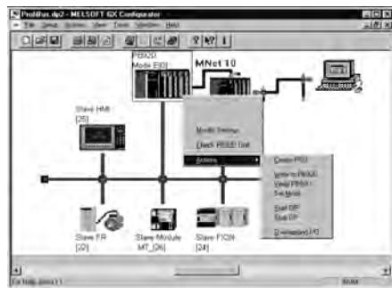
The GX Configurator DP is a user friendly configurations software for the open network PROFIBUS/DP.
