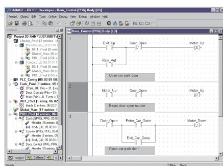
GX IEC Developer provides all functions of the pre-mentioned programs and in addition meets the programming standard: IEC 1131.3 (EN 61131). This makes the software ready for the programming standard of the future and offers beside the FX version in addition the full version as a basis for the on-leading programming of the MELSEC AnS/QnAS series, the MELSEC AnU/QnA series and MELSEC System Q.
