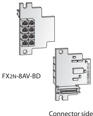
The FX□N-8AV-BD analog setpoint adapters enable the user to set 8 analog setpoint values. The analog values of the potentiometers are read into the controller and used as default setpoint values for timers, counters and data registers by the user's PLC programs. Setpoint value polling and the definition of the potentiometer scales are performed in the PLC program using the dedicated instructions VRRD/VRSC (FNC85/86).
