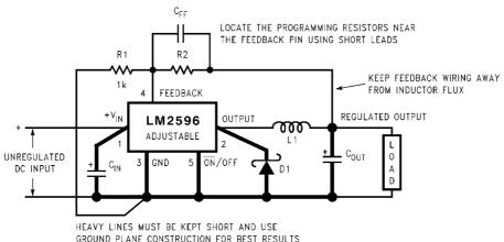
$$V_{OUT} = V_{REF} \left(1 + \frac{R_2}{R_1}\right)$$
