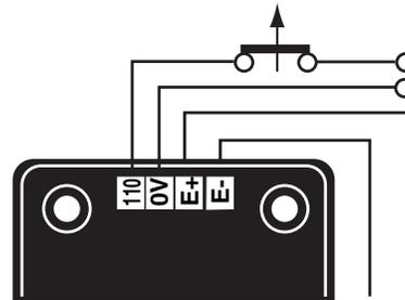
The exciter is switched off by disconnecting the AVR power supply (1 wire - 0 or 110V). Contact rating : 16A - 250V alt.
