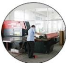
2. Prepare cabinet material by CNC punch
