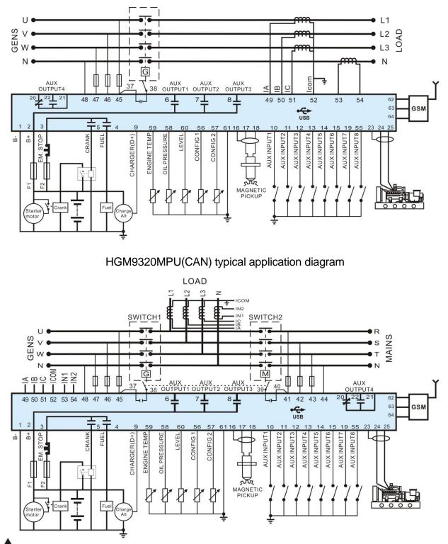
HGM9310MPU(CAN) typical application diagram
