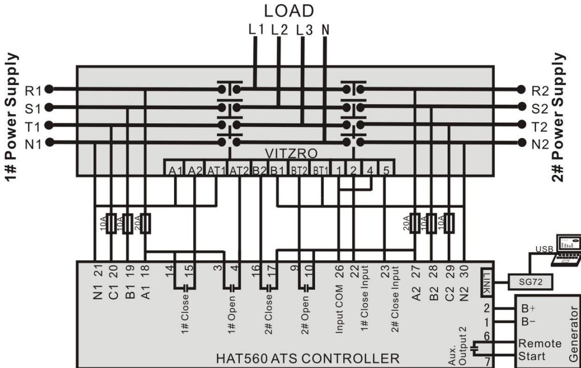
**NOTE:** Set auxiliary output 1 as: 15. 1# Open Output
