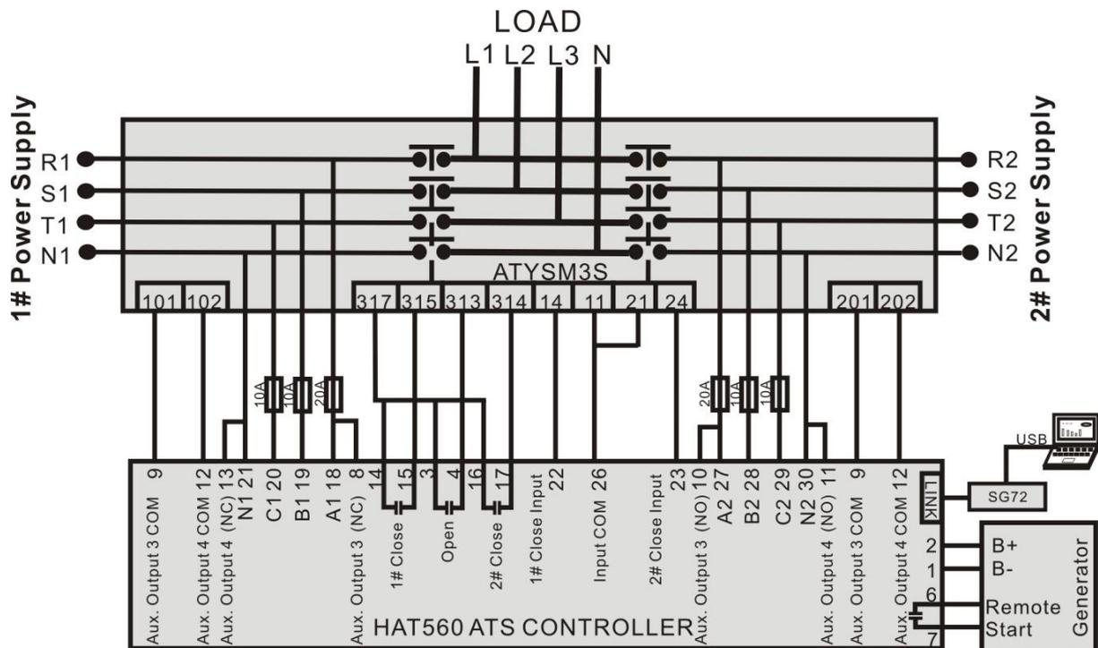
▲Note: The diagram is for reference only. Users should choose proper fuse capacity according to the actual power consumption. If there is no DC power supply, please select "Gen start output (Normally close)".
