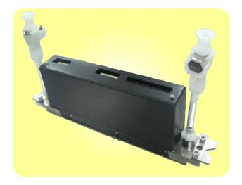
KJ4B-QA06NTB-STDV inkjet printhead is designed for high speed single-pass and multipass applications with water based ink. It delivers 600 dpi × 600 dpi resolution at 75 m/min by making use of 2,656 nozzles arranged across 108 mm width.
