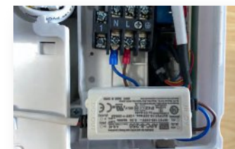
2.Place driver inside A/C power supply box
