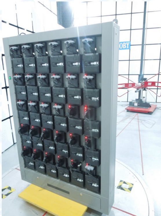
Photo 2 Radiated Emission Test Setup
