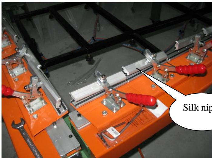
Adjust tighten area according to the dimension of screen frame, then lock the truckle
