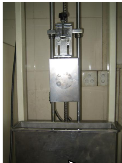
PM-40TC Dipping-type coating machine
