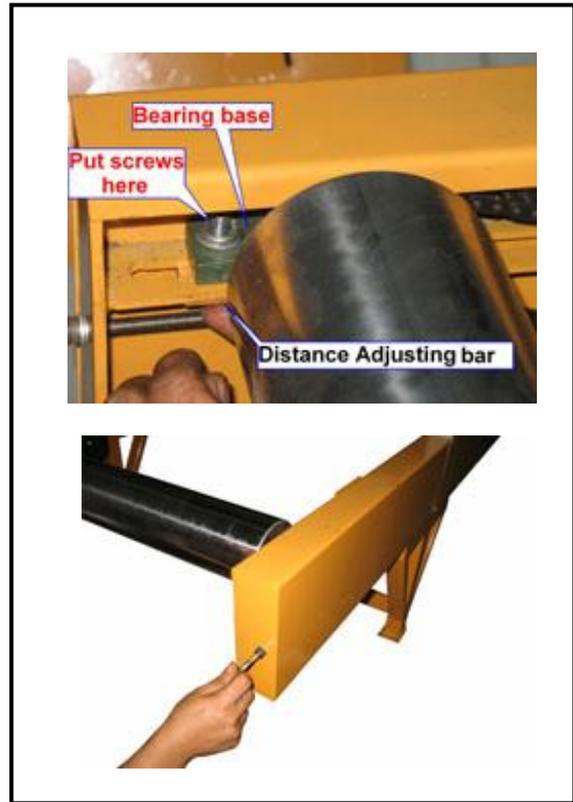
**B/ Assembly “Compliant Roller” to “Outlet Arms”:**
