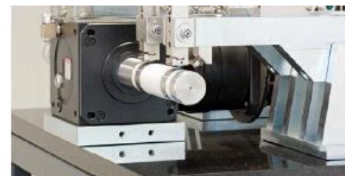
[Wear resistant test in room Temp.]
