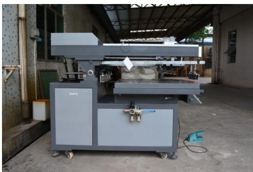
The left side of the machine and the oil-water separator
