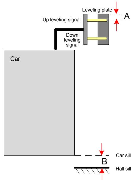
If the car stop position is not fixed at the same floor under different travels or loads, and height deviation between the car position and the hall sill are inconsistent at the same floor, it may be caused by improper speed loop parameters (group F2 parameters). To solve the problem, increase the speed loop proportional gain or decrease the speed loop integral time properly.
