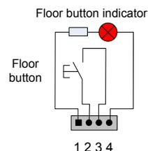
For CCB2, the input signal of JPn corresponds to floor (16+n) button input.
