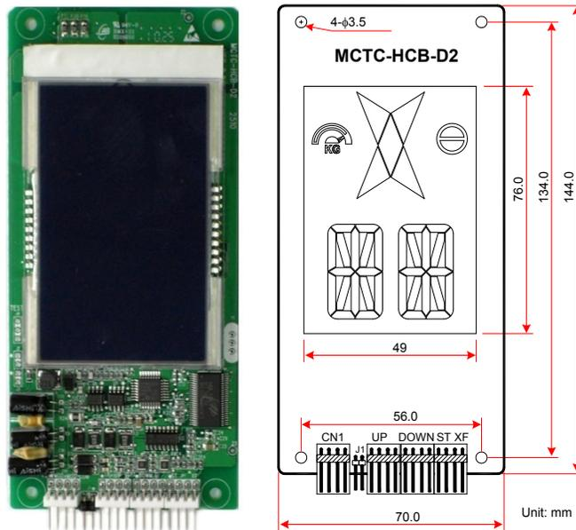
The following figure shows the installation method of HCB-D2.
