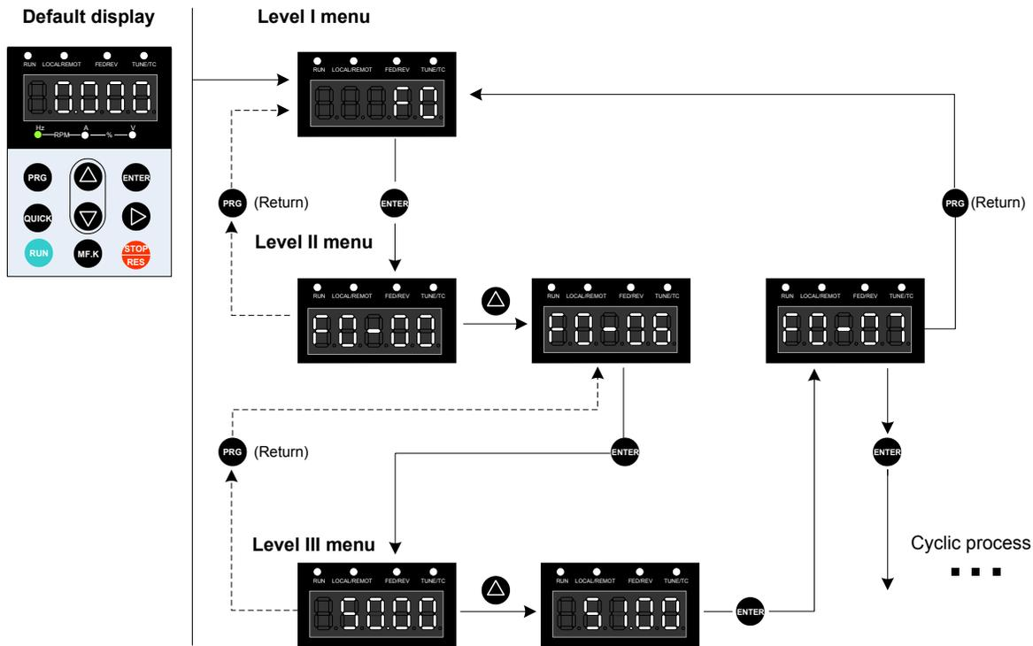
Press to switch the blinking digit.
