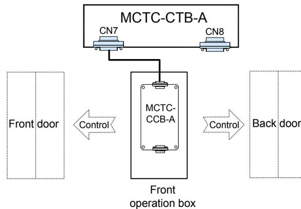
Figure 6-26 CCB wiring of double operation boxes
