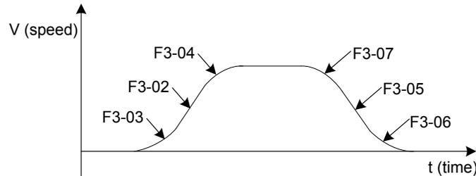
F3-02, F3-03, and F3-04 are used to set the running curve during which the elevator accelerates from startup to the maximum speed. If the acceleration process is too short causing bad riding comfort, decrease the value of F3-02 and increase the values of F3-03 and F3-04 to make the acceleration curve smoother. If the acceleration process is too long, increase the value of F3-02 and decrease the values of F3-03 and F3-04.
