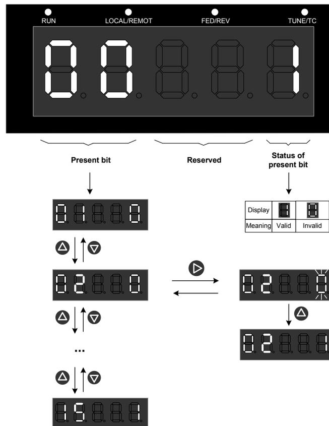
The preceding figure shows that Bit0 is valid, that is, the function defined by Bit0 is enabled.
