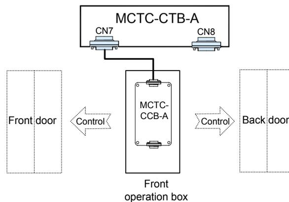
Figure 6-29 CCB wiring of double operation boxes (old method)
