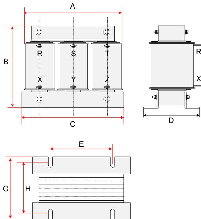
Table 12-2 Physical dimensions of 50–120 A AC reactor
