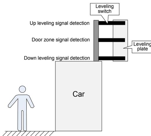
The following table describes the installation requirements of leveling switches
