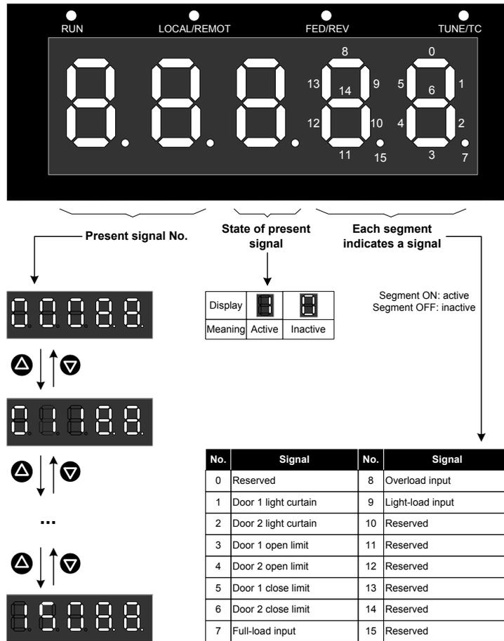
Figure 8-25 FA-34 Car output state
