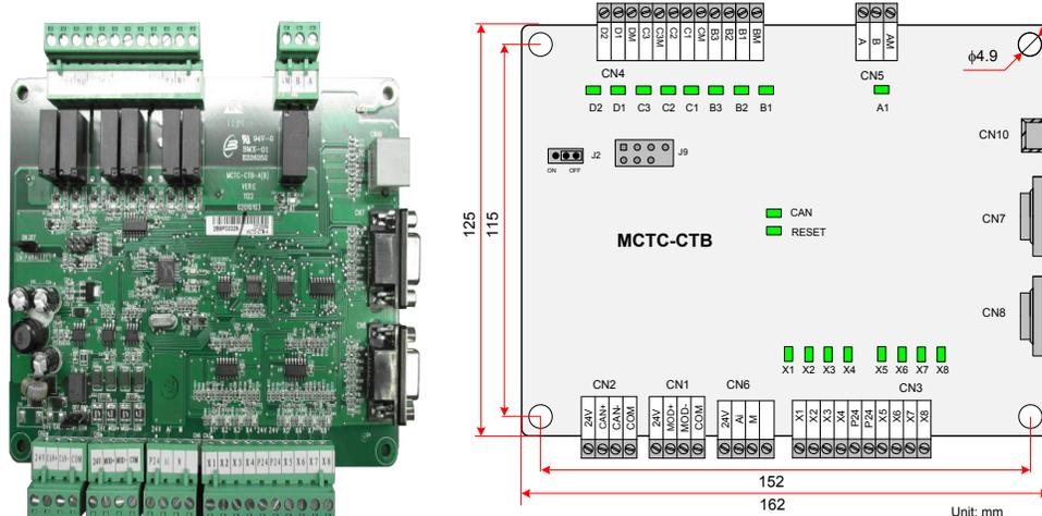
Figure 4-5 Installation method of the CTB (unit: mm)
