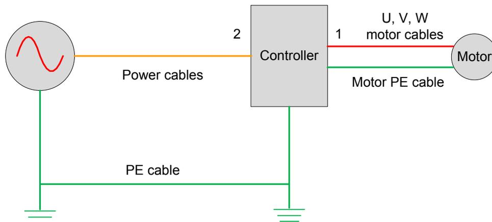
The measures of suppressing interference from the controller are as follows:
