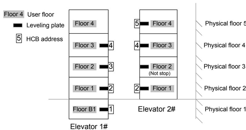
Table 6-10 Parameter setting and HCB addresses of two elevators
