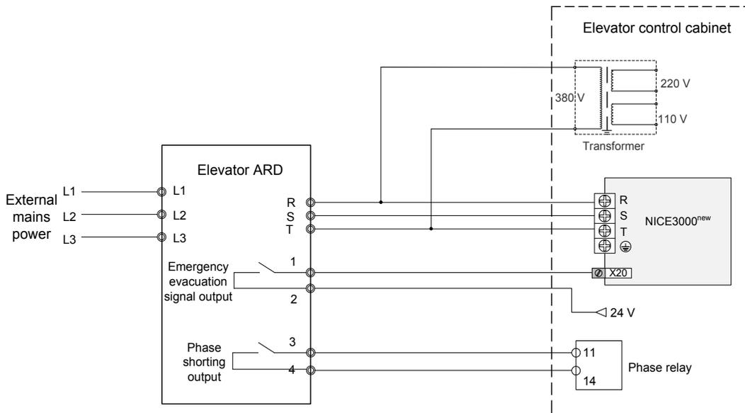
Figure 6-20 Wiring of single-phase (220 V) elevator ARD
