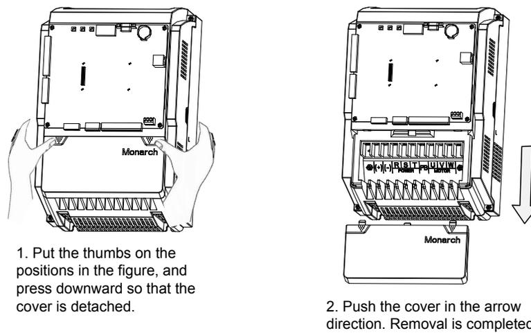
After wiring to the main circuit terminals is completed, reattach the terminal cover.
