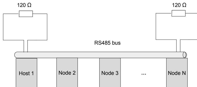
1. The termination resistor can be connected only at two ends of the bus.
