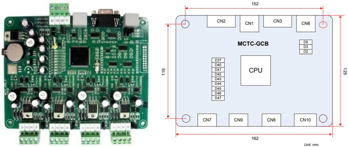
The following figure shows the installation method of the GCB.
