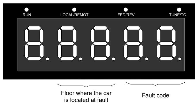
For example, if FC-20 is displayed as **88835**, indicating that the 1st fault code is Err35 and the car is near floor 8 when this fault occurs.
