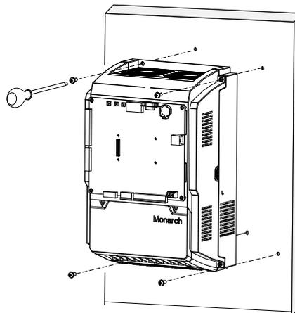
It is forbidden to fasten only the upper two screws, because the controller may fall and be damaged due to uneven force after long-time running. Ensure that all the four screws are fastened.
