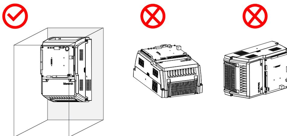
Figure 3-4 Heat dissipation direction
