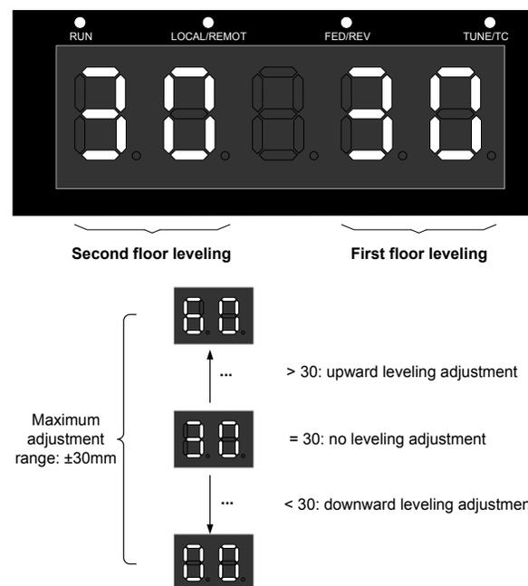
As shown in the preceding figure, the left two LEDs and the right two LEDs respectively show the adjustment bases of the first floor and second floor. If the value is larger than 30, it is upward leveling adjustment; if the value is smaller than 30, it is downward leveling adjustment. The default value "30" indicates that there is no leveling adjustment. The maximum adjustment range is  $\pm 30$  mm.
