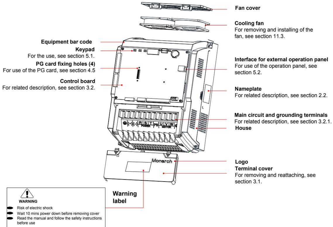
Figure 2-3 Exploded view of the sheet metal structure (18.5–30 kW)
