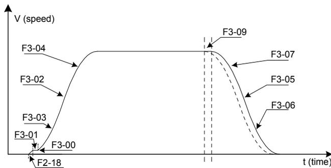
Figure 8-3 Acceleration rate curve
