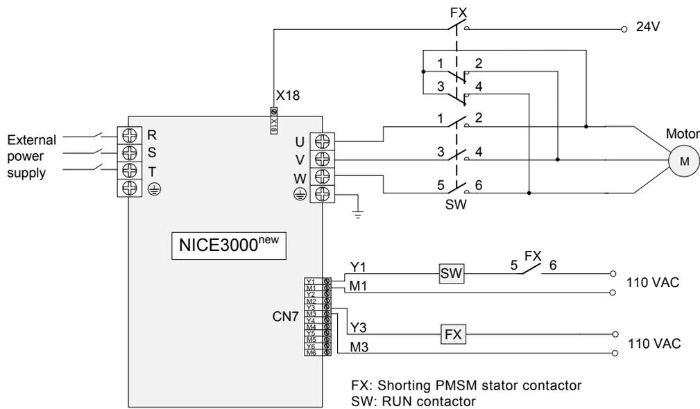
The parameter setting in shorting PMSM stator mode is described in the following table.
