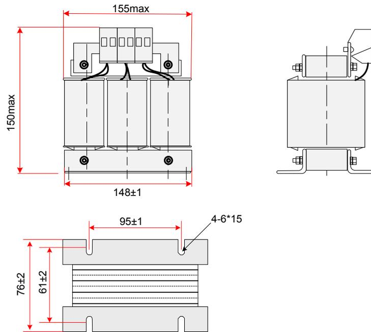
Figure 12-3 Physical dimension diagram of 30–120 A AC input reactor
