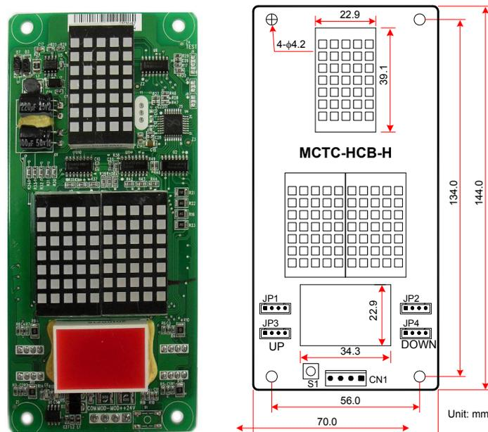
The following figure shows the installation method of HCB-H.
