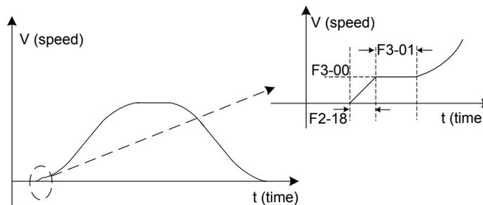
Bad riding comfort due to static friction may often exist in villa elevators. When there is large friction between the guide shoes and the guide rails, large static friction generates at the moment of startup, leading to bad riding comfort. Make the system starts up at the specified speed by setting these parameters to eliminate friction and improve riding comfort.
