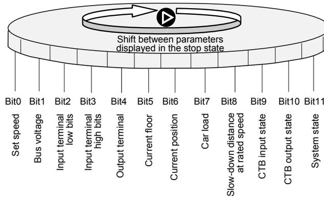
The running and stop parameters of the NICE3000<sup>new</sup> system are the important references for engineers to perform commissioning on site. The parameters are described as follows:
