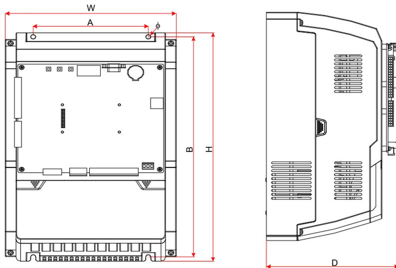
2) Sheet metal structure, 18.5–30 kW, Size-E
