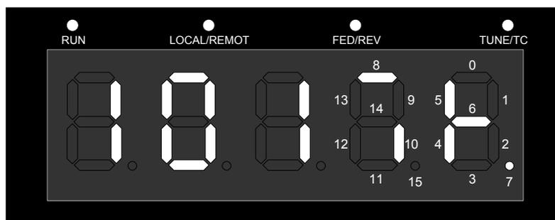
According to the preceding figure, the currently viewed signal 10 (Inspection down) is 1 (Active); besides signal 10, signals 4 (Safety circuit feedback), 5 (Door lock circuit feedback), 6 (RUN contactor feedback), 7 (Brake contactor feedback), and 8 (Inspection signal) are active.
