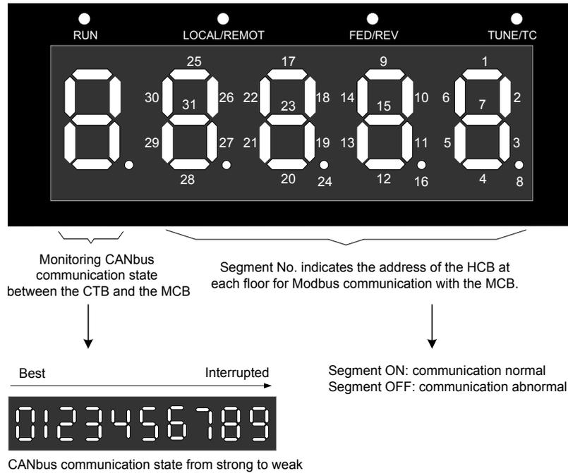
For example, if the LEDs are shown as the following figure, it indicates that Modbus communication of addresses 1, 5, 6, 7, 12, 15, 16, 18, 19, 21, 22, 23, 25, 26 and 27 is abnormal, and Modbus communication of other addresses is normal. CANbus communication state displayed by the LED is 3, indicating normal communication.
