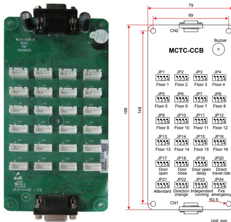
The following figure shows the installation method of the CCB.
