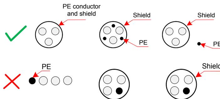
To suppress emission and conduction of the radio frequency interference effectively, the shield of the shielded cable is copper braid. The braided density of the copper braid should be greater than 90% to enhance the shielding efficiency and conductivity, as shown in the following figure.
