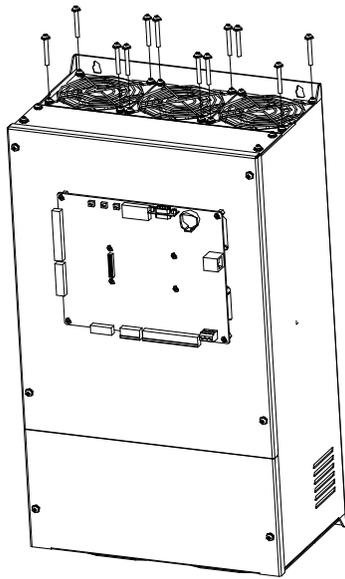
2. Lift the fan cover and fan a little, and disconnect the fan power cable from the socket.
