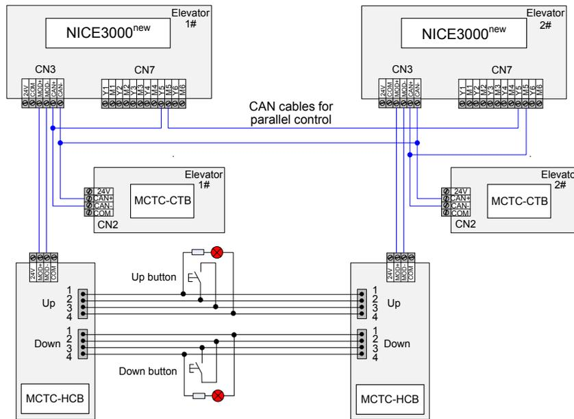
2. Alternative parallel control scheme (CAN2 communication port CN4)
