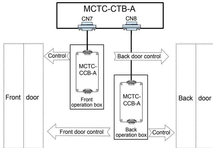
The following figure shows the CCB wiring of modes 4.
