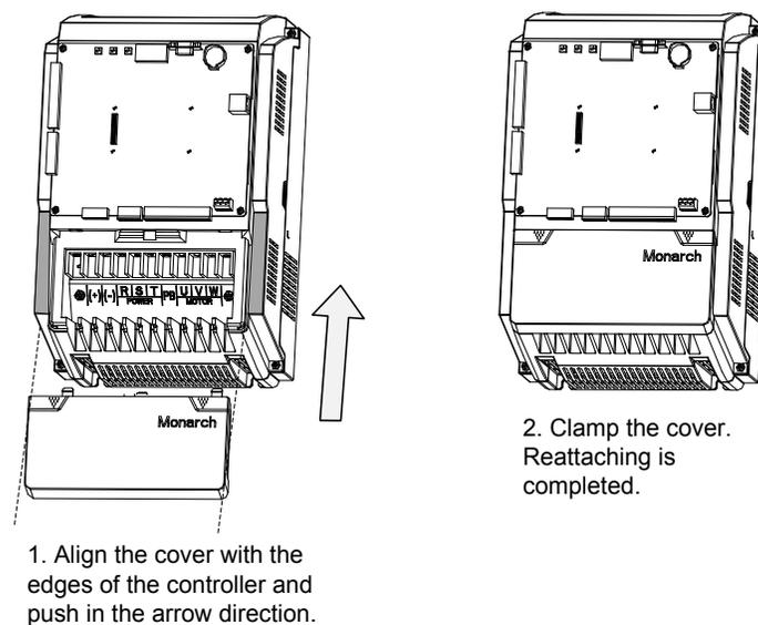
2. Removing and reattaching the terminal cover with sheet metal structure
