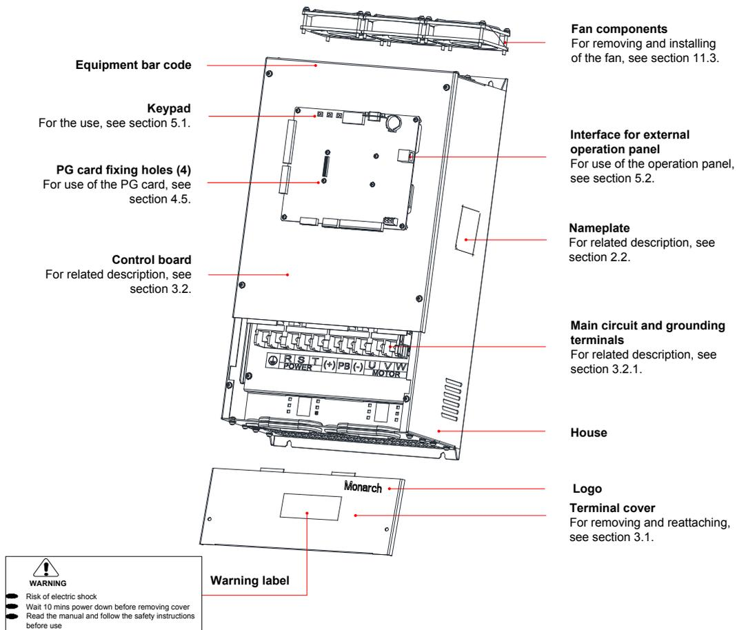
Figure 2-4 Exploded view of the sheet metal structure (37–55 kW)
