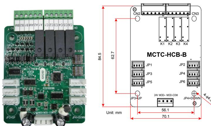
The following figure shows the installation method of HCB-B.
