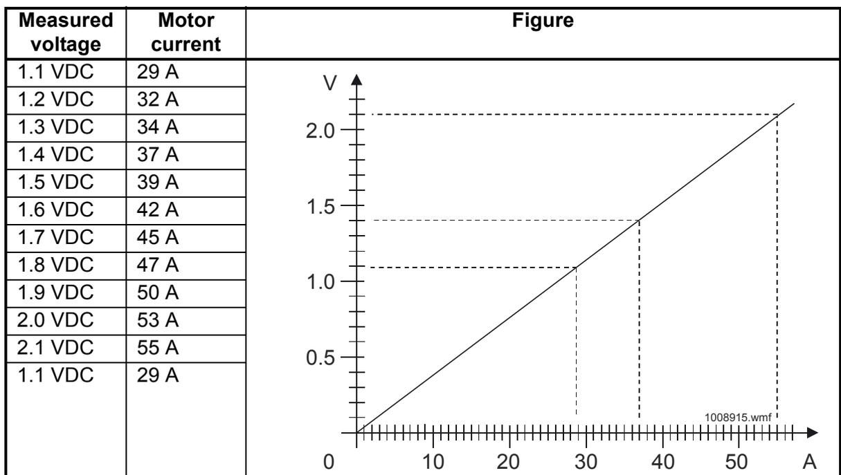
**6.7 Balance measurement in elevators with V<sup>3</sup>F25 drive**
