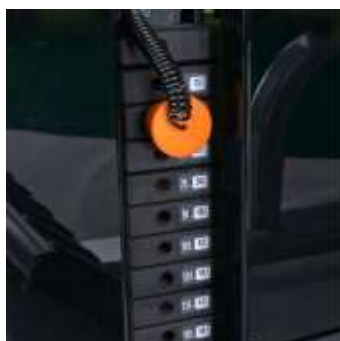
Safe Magnetic Pin 磁性安全选片插销
