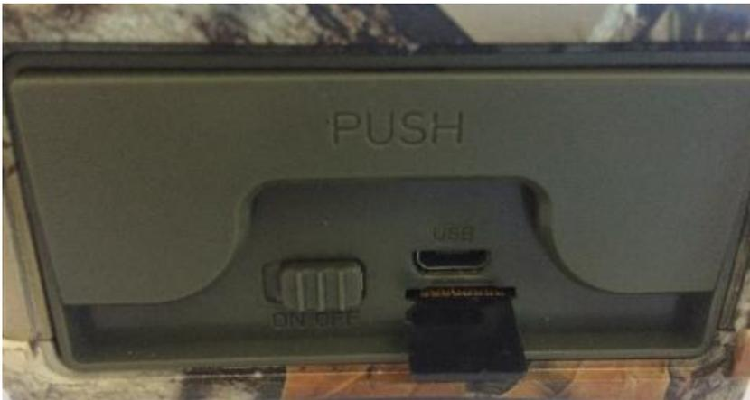
C: Put the switch to “ON” position, and the indicator light will flashing 3 times to go out, Camera will enter PIR detect status.
