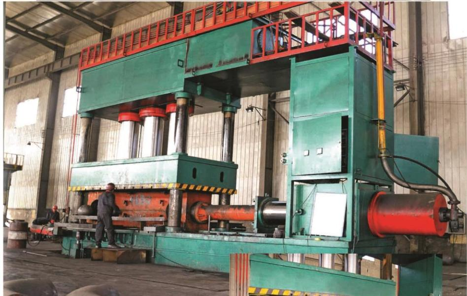
▲ 不锈钢弯头推制机 Stainless Steel Elbow Pushing Machine
