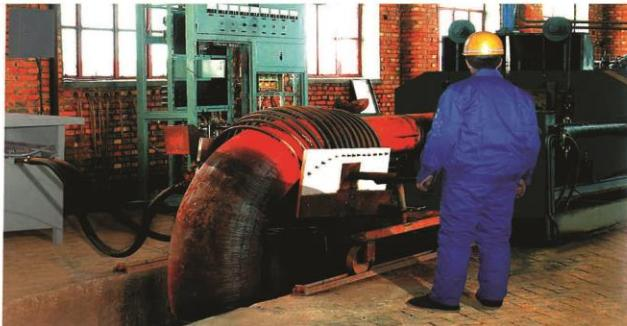
▲ 弯头推制机 Elbow Pushing Machine
