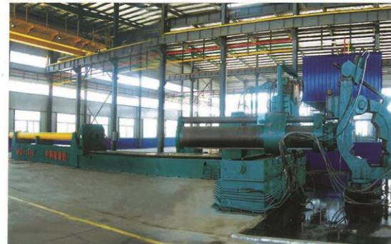
▲ 中频弯管推制机 Intermediate Frequency Bent Pipe Pushing Machine
