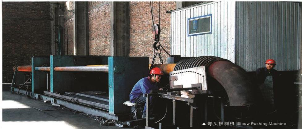
▲ 弯头推制机 Elbow Pushing Machine
