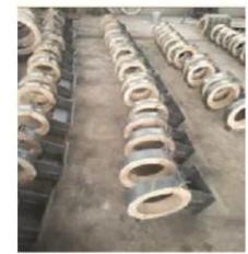
隔热管托 Insulated pipe holder
