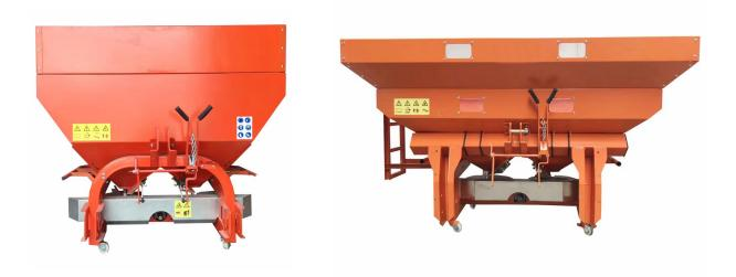
Tractor mounted type fertilizer spreader (1000-2000 L)
