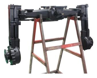
Configuration the Drive axle standard width is 1.5m, and also can custom design 1.8m. (www.walijixie.com)
