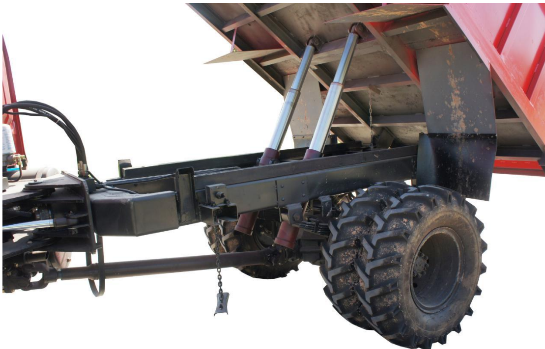
Dual hydraulic cylinder dump
