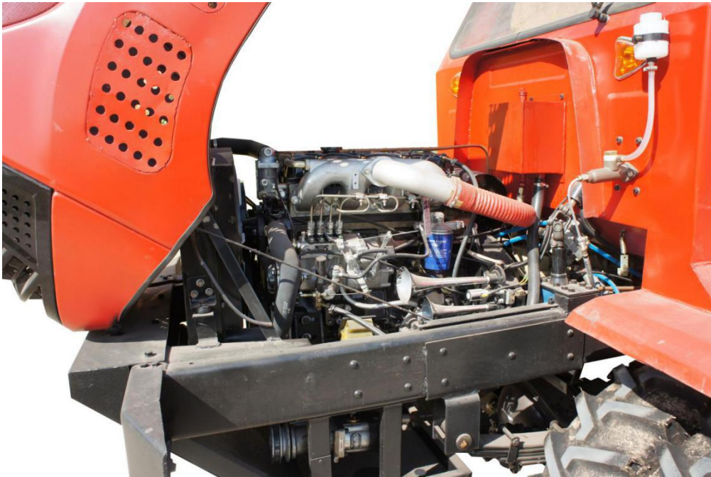
Yunnei 4100QB 4 cylinder water-cooled diesel engine with 90 HP.
