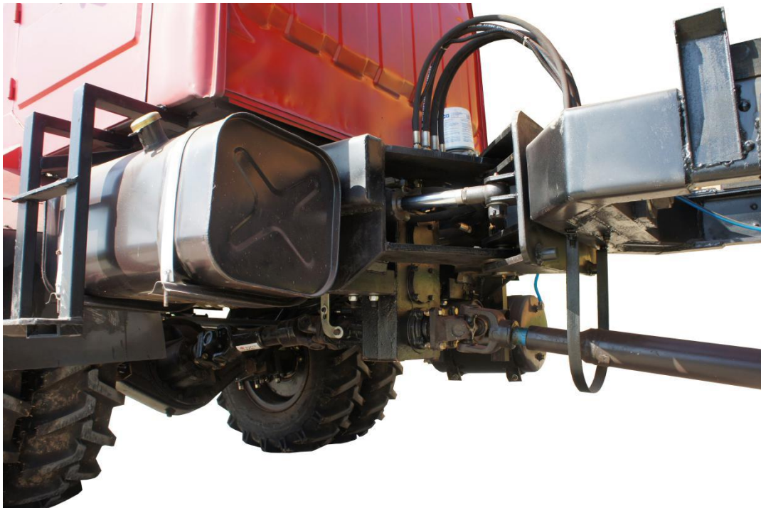
Configuration the High and Low Speed Gearbox + articulated steer System
