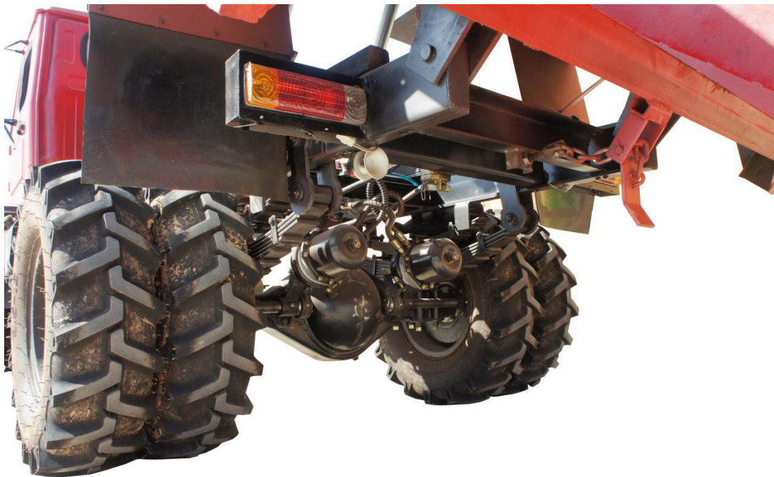
The front and rear axles are equipped with air-breaking brakes
