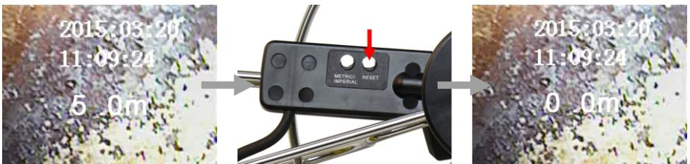
2. Press the "RESET" button to reset the value of cable length
