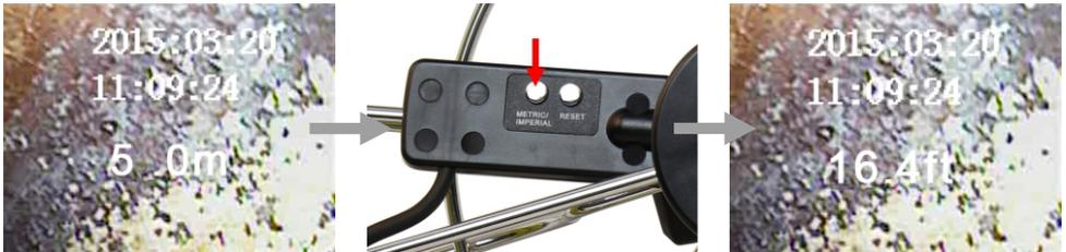
1. Press the "METRIC/IMPERIAL" button to alternate metric and imperial unit
