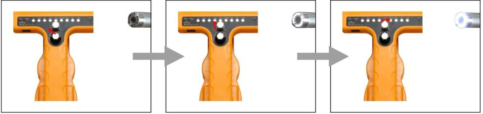
1. Rotate the brightness adjustment knob in a clockwise direction, the LEDs will become more and more bright
