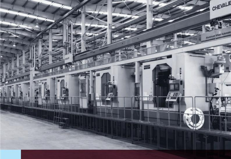
New intelligent gantry-type automatic aluminum wheel production equipment
