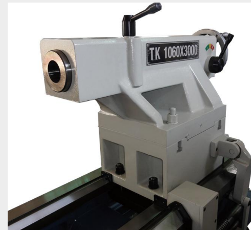
Heavy duty cast iron tailstock body
