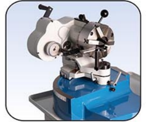
Patent No. 135236 Double cams. It can grind tool of 1/2/3/4/6 Flutes.
