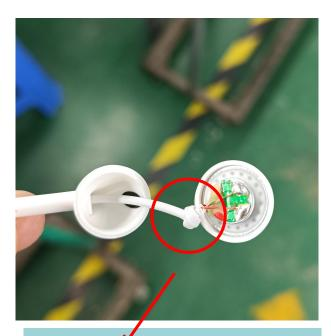
Tie a knot at the end of wire to enforce pull durability
