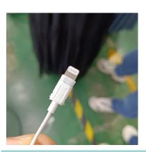
Injection to enforce the plug & pull & bend
