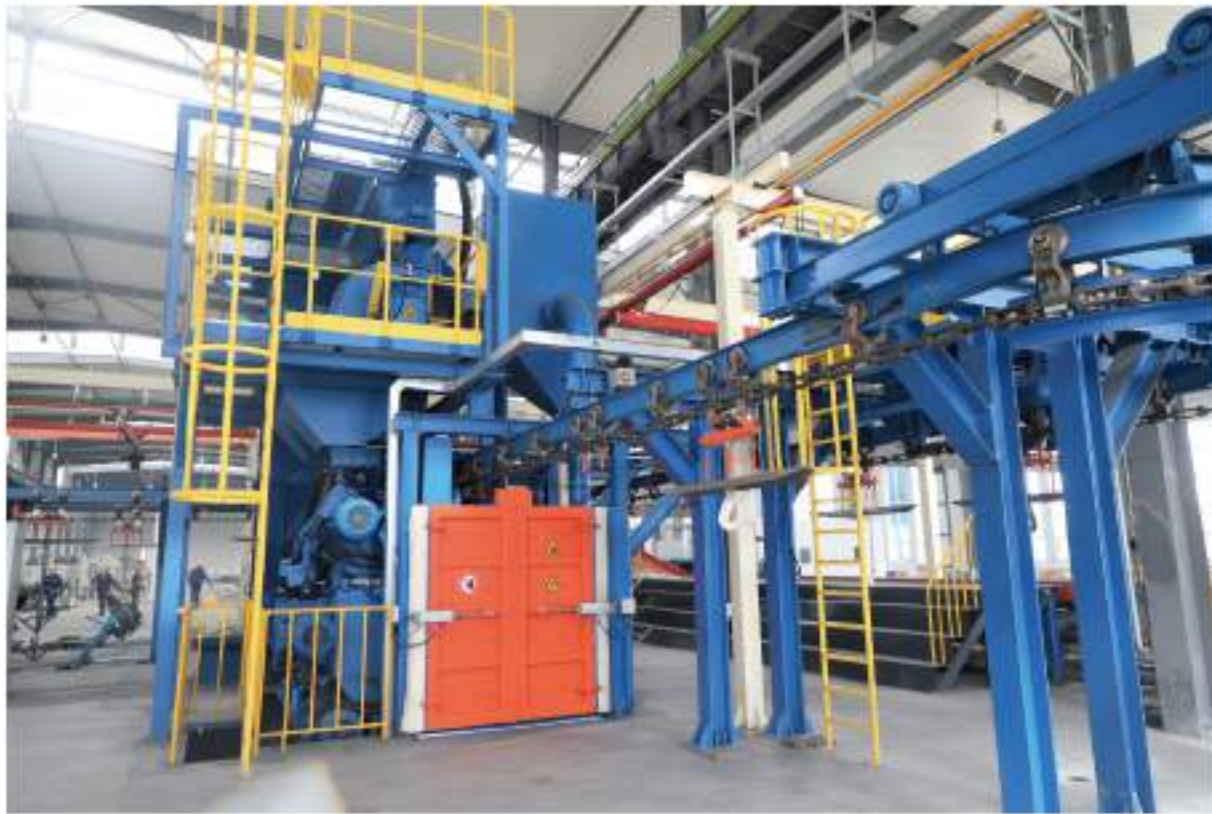
3 suspended shot blasting machines Production efficiency: 36 tons per hour
