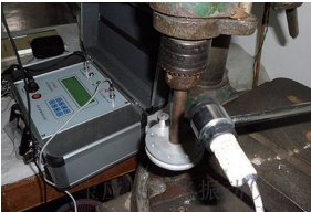
Measurement of rotating speed of machinery and equipment
