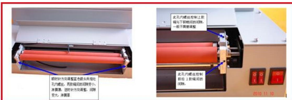
7) If not to use the machine for long time, you'd better clear rubber rollers before you store it. Pull the alcohol into the storage tank to replace the glossy oil, and keep the machine working for a while. Or open the cap of the rubber roller, pull the alcohol between the 2 rollers, keep the rollers work for a while, or use a piece of cotton with alcohol clean the rubber roller.
