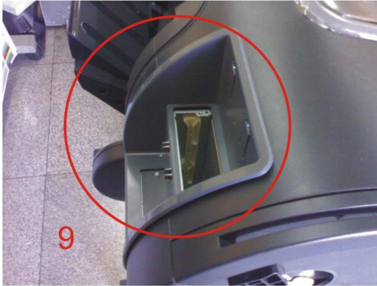
2-10. Take down the shelf of the printing card (within the red circle)
