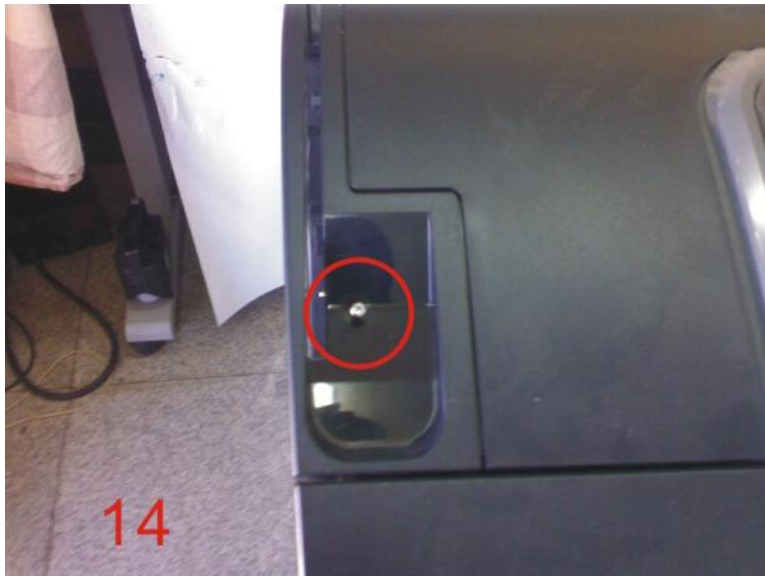
2-15. Take out the front baffle of the machine, take out the screw ( in the red circle)
