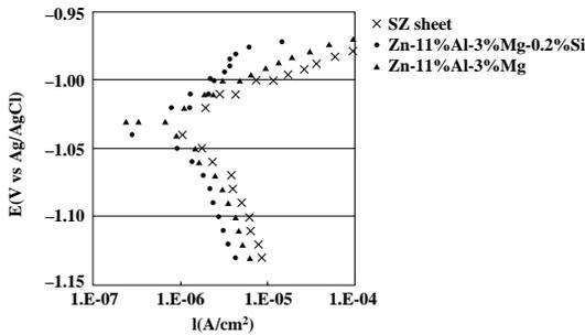
Fig. 8 Polarization after 3-h immersion in 5% NaCl solution
