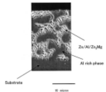
Fig. 6 Sectional micrograph of Zn-11%Al-3%Mg-0.2%Si-plated sheet
