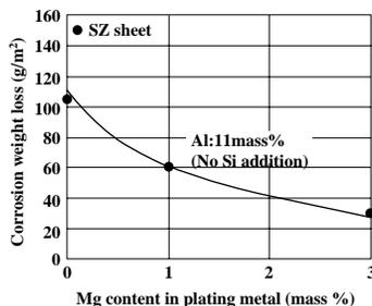
Fig. 3 Influence of Mg content in plating metal on corrosion weight loss at 500-h SST
