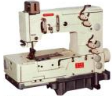
JG-1826 雙針四回縫外曲牙機 2-needle 4-point(3-step)zizzag picoting machine
