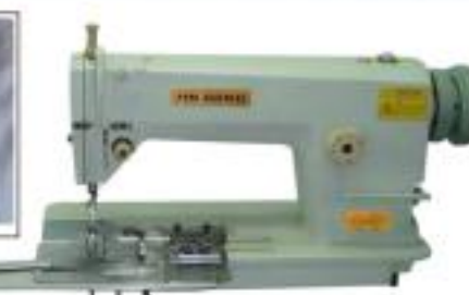
JG-1836-1 單針平車打條機 Single needle pin-tuck machine
