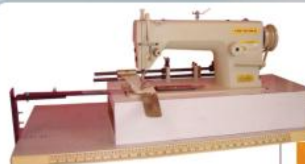
JG-1836 單針平車打條機 Single needle pin-tuck machine
