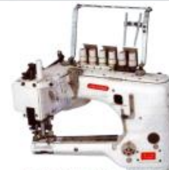
JG-36200 4針曲臂型卷接繡機 Chain stitch feed-off arm machine
