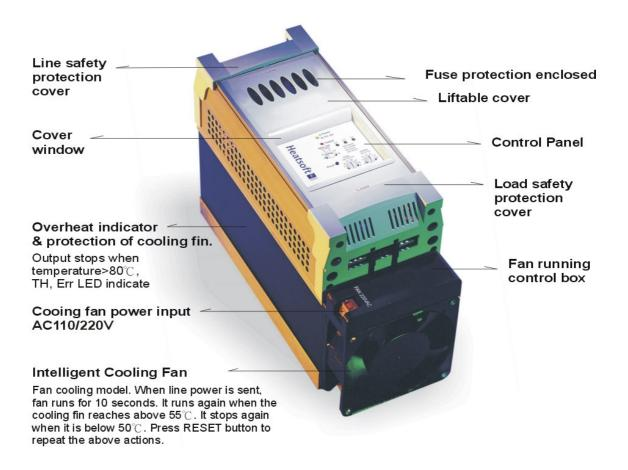
**Note:** The cover can be lifted by pushing the load safety protection cover downwards. For wiring and fuse changing, if it is necessary, the aluminum side-on on top can be pulled open and away down the cover.
