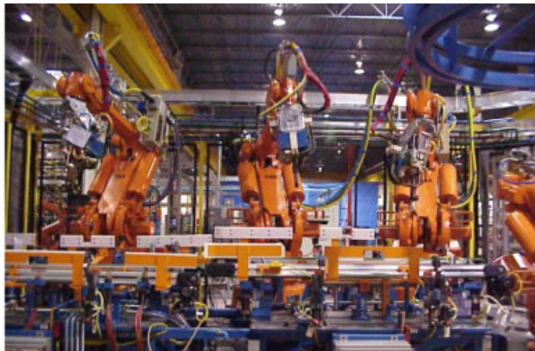
Robotic welding on aluminium body assembly line
