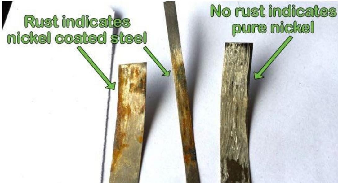
Fun fact: I actually discovered Method 1 while preparing to test out my idea for Method 2. I used a rotary tool with a sanding wheel to scuff up some sample strips so I could put them in saltwater. That's when I realized that some of the strips were throwing sparks. By completing the saltwater test, I confirmed my suspicion that it was the steel core strips that were shooting sparks while the pure nickel strips didn't spark at all.
