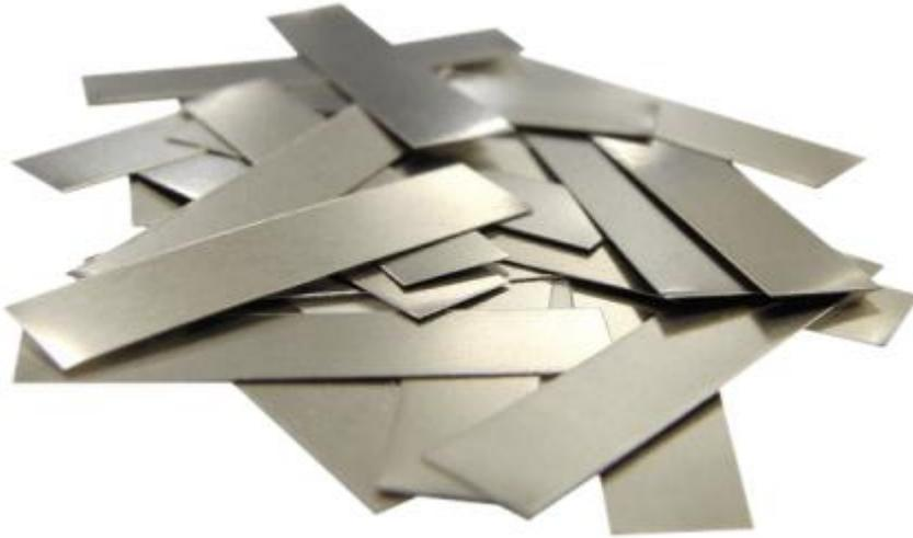
Building your own electric bicycle battery isn't rocket science, but it isn't the simplest job either. When putting together an ebike battery pack, you want to make sure you're using pure nickel strips and not nickel coated steel strips.
