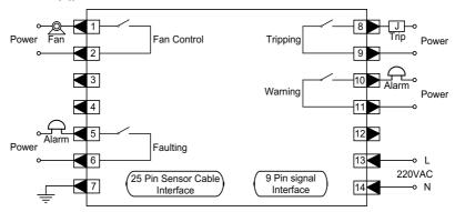
LD-B10-10DP(B)/EP(B)/FP(B) wiring diagram (Note: 9-pin interface is not available for LD-B10-10DP(B))
