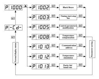
**Note 1:** When the meter is displaying the function prompts, press key SET to enter into the corresponding data display window. If there are multiple function parameters, each parameter is set by pressing the key SET in turn.
