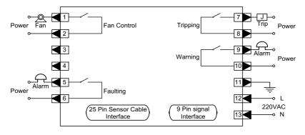
LD-B10-10DP/EP/FP wiring diagram (Note: 9-pin interface is not available for
