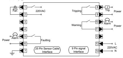
Note 1: D25 sensor cable is connected to Pt100 and PTC (type C) signal input; D9 signal cable is connected to RS485 signal (type F) and 4~20mA current signal (type E) output.
