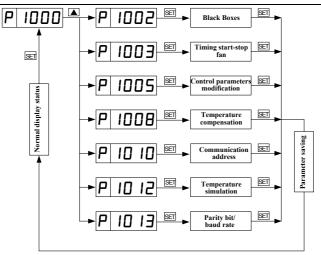
**Note 1:** When the meter is displaying the function prompts, press key SET to enter into the corresponding data display window. If there are multiple function parameters, each parameter is set by pressing the key SET in turn.
