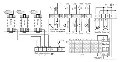
Notes: The terminal with "JP7" and without cables is a standby terminal. There is no definition for the standby terminal.
