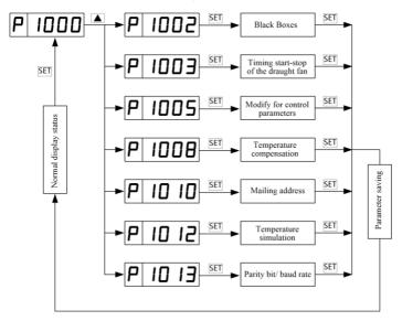
**Note 1:** When displaying the function prompts, press SET key to enter into the corresponding data display window; and with multiple function parameters, repeat pressing the SET key to set up from the larger numbers from the lower serial number.
