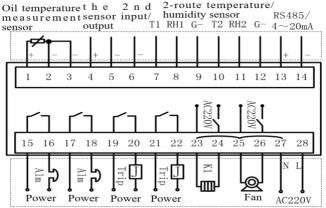
Terminals 1-6 are 2-route PT100 sensor connecting terminals. 1 and 4 are positive terminals. And 4, 5 and 6 (connected in parallel) are output.
